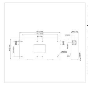
RF Solution offer a wide selection of Dual Junction Isolator for global customers. UIYCDI16080A is a Dual Junction Isolator in Frequency Range of 10~55 MHz. It is made of high quality materials under a high standard, the Bandwidth Max of this product is 20%, Insertion Loss Max is 2.40~7.00 dB and Isolation Min is 24.0~40.0 dB. The component has a good working performance and stability, it is ideal for handling a Forward Power of 50 W.
