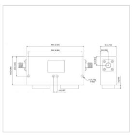
RF Solution offer a wide selection of Dual Junction Isolator for global customers. UIYCDI6432A is a Dual Junction Isolator in Frequency Range of  $700\sim3500$  MHz. It is made of high quality materials under a high standard, the Bandwidth Max of this product is 20%, Insertion Loss Max is  $0.60\sim1.00$  dB and Isolation Min is  $40.0\sim50.0$  dB. The component has a good working performance and stability, it is ideal for handling a Forward Power of 100/150/200 W.
