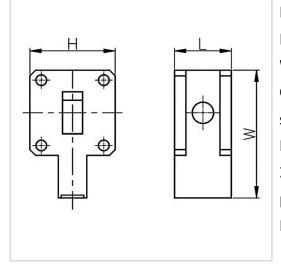
RF Solution offer a wide selection of Waveguide Isolator for global customers. BG1034-WR140 is a Waveguide Isolator in Frequency Range of 13.9~14.3 GHz. It is made of high quality materials under a high standard, the Bandwidth Max of this product is 100%, Insertion Loss Max is 0.50 dB and Isolation Min is 21.0 dB. The component has a good working performance and stability, it is ideal for handling a Forward Power of /.
