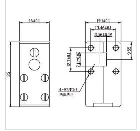
RF Solution offer a wide selection of Waveguide Isolator for global customers. BG1635-WR28 is a Waveguide Isolator in Frequency Range of 34.0~36.0 GHz. It is made of high quality materials under a high standard, the Bandwidth Max of this product is 100%, Insertion Loss Max is 0.25 dB and Isolation Min is 18.0 dB. The component has a good working performance and stability, it is ideal for handling a Forward Power of /.
