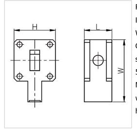
RF Solution offer a wide selection of Waveguide Isolator for global customers. BG2151-WR62 is a Waveguide Isolator in Frequency Range of 12.0~18.0 GHz. It is made of high quality materials under a high standard, the Bandwidth Max of this product is 5%/10%, Insertion Loss Max is 0.30 dB and Isolation Min is 23.0~25.0 dB. The component has a good working performance and stability, it is ideal for handling a Forward Power of /.
