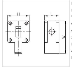
RF Solution offer a wide selection of Waveguide Isolator for global customers. BG2552-WR75 is a Waveguide Isolator in Frequency Range of 10.0~15.0 GHz. It is made of high quality materials under a high standard, the Bandwidth Max of this product is 5%/10%, Insertion Loss Max is 0.25~0.30 dB and Isolation Min is 23.0~25.0 dB. The component has a good working performance and stability, it is ideal for handling a Forward Power of /.
