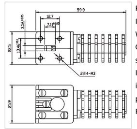
RF Solution offer a wide selection of Waveguide Isolator for global customers. BG2660-WR28 is a Waveguide Isolator in Frequency Range of 26.0~40.0 GHz. It is made of high quality materials under a high standard, the Bandwidth Max of this product is 100%, Insertion Loss Max is 0.40~0.45 dB and Isolation Min is 16.0~20.0 dB. The component has a good working performance and stability, it is ideal for handling a Forward Power of /.
