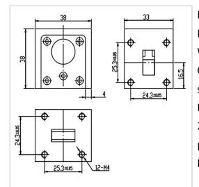
RF Solution offer a wide selection of Waveguide Isolator for global customers. BG3838-WR140 is a Waveguide Isolator in Frequency Range of 15.0~18.0 GHz. It is made of high quality materials under a high standard, the Bandwidth Max of this product is 100%, Insertion Loss Max is 0.40 dB and Isolation Min is 20.0 dB. The component has a good working performance and stability, it is ideal for handling a Forward Power of /.
