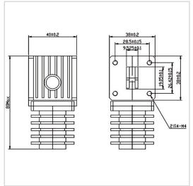
RF Solution offer a wide selection of Waveguide Isolator for global customers. BG4080-WR75 is a Waveguide Isolator in Frequency Range of 13.7~14.7 GHz. It is made of high quality materials under a high standard, the Bandwidth Max of this product is 100%, Insertion Loss Max is 0.25 dB and Isolation Min is 20.0 dB. The component has a good working performance and stability, it is ideal for handling a Forward Power of /.
