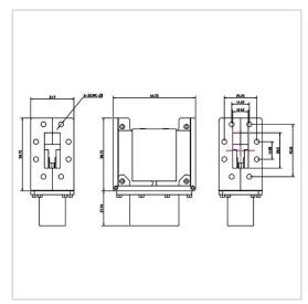
RF Solution offer a wide selection of Waveguide Isolator for global customers. BG6658-WR112 is a Waveguide Isolator in Frequency Range of 18.0~26.5 GHz. It is made of high quality materials under a high standard, the Bandwidth Max of this product is 100%, Insertion Loss Max is 0.20 dB and Isolation Min is 20.0 dB. The component has a good working performance and stability, it is ideal for handling a Forward Power of 100 W.
