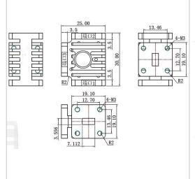
RF Solution offer a wide selection of Waveguide Circulator for global customers. BH2530-WR28 is a Waveguide Circulator in Frequency Range of 26.5~40.0 GHz. It is made of high quality materials under a high standard, the Bandwidth Max of this product is 100%, Insertion Loss Max is 0.35 dB and Isolation Min is 15.0 dB. The component has a good working performance and stability, it is ideal for handling a Forward Power of /.
