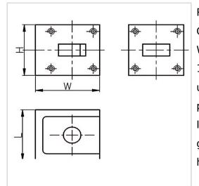
RF Solution offer a wide selection of Waveguide Circulator for global customers. BH3036-WR51 is a Waveguide Circulator in Frequency Range of 14.5~22.0 GHz. It is made of high quality materials under a high standard, the Bandwidth Max of this product is 5/10%, Insertion Loss Max is 0.30 dB and Isolation Min is 23.0~25.0 dB. The component has a good working performance and stability, it is ideal for handling a Forward Power of /.
