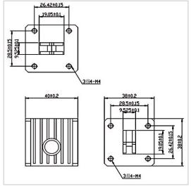
RF Solution offer a wide selection of Waveguide Circulator for global customers. BH4038-WR75 is a Waveguide Circulator in Frequency Range of 10.0~15.0 GHz. It is made of high quality materials under a high standard, the Bandwidth Max of this product is 100%, Insertion Loss Max is 0.30 dB and Isolation Min is 18.0 dB. The component has a good working performance and stability, it is ideal for handling a Forward Power of /.
