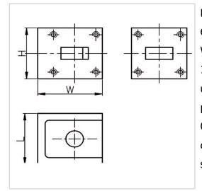
RF Solution offer a wide selection of Waveguide Circulator for global customers. BH4444-WR75 is a Waveguide Circulator in Frequency Range of 10.0~15.0 GHz. It is made of high quality materials under a high standard, the Bandwidth Max of this product is 5/10/100%, Insertion Loss Max is 0.25~0.30 dB and Isolation Min is 23.0~25.0 dB. The component has a good working performance and stability, it is ideal for handling a Forward Power of /.
