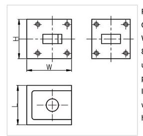
RF Solution offer a wide selection of Waveguide Circulator for global customers. BH4648-WR90 is a Waveguide Circulator in Frequency Range of 8.0~12.4 GHz. It is made of high quality materials under a high standard, the Bandwidth Max of this product is 20%, Insertion Loss Max is 0.25 dB and Isolation Min is 23.0 dB. The component has a good working performance and stability, it is ideal for handling a Forward Power of /.
