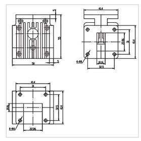
RF Solution offer a wide selection of Waveguide Circulator for global customers. BH5055-WR90 is a Waveguide Circulator in Frequency Range of 9.0~9.55 GHz. It is made of high quality materials under a high standard, the Bandwidth Max of this product is 100%, Insertion Loss Max is 0.35 dB and Isolation Min is 20.0 dB. The component has a good working performance and stability, it is ideal for handling a Forward Power of /.
