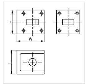
RF Solution offer a wide selection of Waveguide Circulator for global customers. BH6880-WR137 is a Waveguide Circulator in Frequency Range of 5.4~8.0 GHz. It is made of high quality materials under a high standard, the Bandwidth Max of this product is 20%, Insertion Loss Max is 0.25 dB and Isolation Min is 25.0 dB. The component has a good working performance and stability, it is ideal for handling a Forward Power of /.
