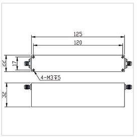
RF Solution offer a wide selection of Band Stop Filter for global customers. BSF-2110M2155A-S is a Band Stop Filter in Rejection Band of 2110~2115 MHz. It is made of high quality materials under a high standard, the Pass Band of this product is DC~2095MHz / 2170~4200MHz, Insertion Loss Max is 1.8 dB and Rejection Min is 40 dB. The component has a good working performance and stability, it is ideal for handling a Rated Power of 20 W.
