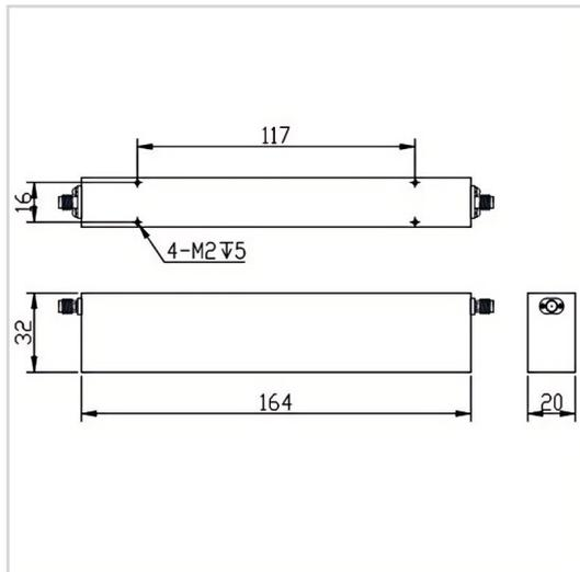
RF Solution offer a wide selection of Band Stop Filter for global customers. BSF-2200M2600A-S is a Band Stop Filter in Rejection Band of 2200~2600 MHz. It is made of high quality materials under a high standard, the Pass Band of this product is DC~2150MHz / 2650~8000MHz, Insertion Loss Max is 2.5 dB and Rejection Min is 50 dB. The component has a good working performance and stability, it is ideal for handling a Rated Power of 50 W.
