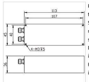
RF Solution offer a wide selection of Band Stop Filter for global customers. BSF-2300M2400A-N is a Band Stop Filter in Rejection Band of 2273~2400 MHz. It is made of high quality materials under a high standard, the Pass Band of this product is DC~2273MHz / 2427~6000MHz, Insertion Loss Max is 2.0 dB and Rejection Min is 50 dB. The component has a good working performance and stability, it is ideal for handling a Rated Power of 10 W.
