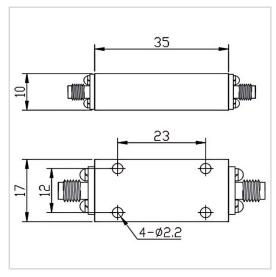
RF Solution offer a wide selection of Band Stop Filter for global customers. BSF-24G24.25A-S is a Band Stop Filter in Rejection Band of 24.0~24.25 GHz. It is made of high quality materials under a high standard, the Pass Band of this product is DC~23GHz / 25.25~40GHz, Insertion Loss Max is 3.0 dB and Rejection Min is 40 dB. The component has a good working performance and stability, it is ideal for handling a Rated Power of 1 W.
