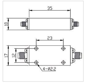
RF Solution offer a wide selection of Band Stop Filter for global customers. BSF-26.5G29.5A-S is a Band Stop Filter in Rejection Band of 26.5~29.5 GHz. It is made of high quality materials under a high standard, the Pass Band of this product is DC~25GHz / 31~50GHz, Insertion Loss Max is 3.0 dB and Rejection Min is 60 dB. The component has a good working performance and stability, it is ideal for handling a Rated Power of 1 W.
