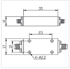
RF Solution offer a wide selection of Band Stop Filter for global customers. BSF-27.5G28.35A-S is a Band Stop Filter in Rejection Band of 27.5~28.35 GHz. It is made of high quality materials under a high standard, the Pass Band of this product is DC~26.3GHz / 29.55~50GHz, Insertion Loss Max is 3.0 dB and Rejection Min is 60 dB. The component has a good working performance and stability, it is ideal for handling a Rated Power of 1 W.
