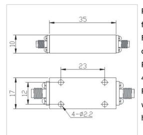
RF Solution offer a wide selection of Band Stop Filter for global customers. BSF-37G40A-S is a Band Stop Filter in Rejection Band of 37.0~40.0 GHz. It is made of high quality materials under a high standard, the Pass Band of this product is DC~35.5GHz / 41.5~50GHz, Insertion Loss Max is 3.0 dB and Rejection Min is 60 dB. The component has a good working performance and stability, it is ideal for handling a Rated Power of 1 W.
