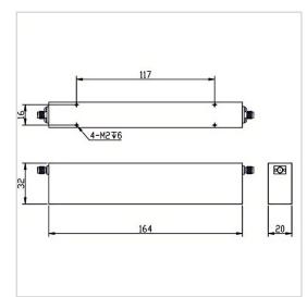
RF Solution offer a wide selection of Band Stop Filter for global customers. BSF-3850M4200A-S is a Band Stop Filter in Rejection Band of 3850~4200 MHz. It is made of high quality materials under a high standard, the Pass Band of this product is DC~3820MHz / 4230~8000MHz, Insertion Loss Max is 3.0 dB and Rejection Min is 40 dB. The component has a good working performance and stability, it is ideal for handling a Rated Power of 20 W.
