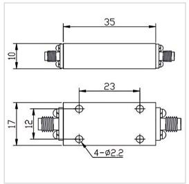
RF Solution offer a wide selection of Band Stop Filter for global customers. BSF-39.5G43.5A-S is a Band Stop Filter in Rejection Band of 39.5~43.5 GHz. It is made of high quality materials under a high standard, the Pass Band of this product is DC~38GHz / 45~50GHz, Insertion Loss Max is 3.0 dB and Rejection Min is 40 dB. The component has a good working performance and stability, it is ideal for handling a Rated Power of 1 W.
