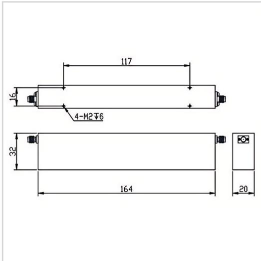
RF Solution offer a wide selection of Band Stop Filter for global customers. BSF-4400M5000A1-S is a Band Stop Filter in Rejection Band of 4400~5000 MHz. It is made of high quality materials under a high standard, the Pass Band of this product is DC~4340MHz / 5060~8000MHz, Insertion Loss Max is 3.0 dB and Rejection Min is 40 dB. The component has a good working performance and stability, it is ideal for handling a Rated Power of 20 W.
