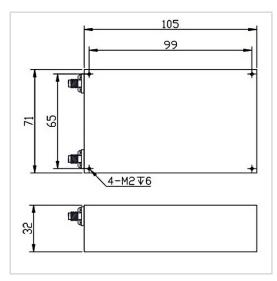
RF Solution offer a wide selection of Band Stop Filter for global customers. BSF-4400M5000A2-S is a Band Stop Filter in Rejection Band of 4400~5000 MHz. It is made of high quality materials under a high standard, the Pass Band of this product is DC~4340MHz / 5060~8000MHz, Insertion Loss Max is 3.0 dB / 5.0 dB and Rejection Min is 80 dB. The component has a good working performance and stability, it is ideal for handling a Rated Power of 10 W.
