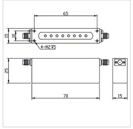
RF Solution offer a wide selection of Band Stop Filter for global customers. BSF-5400M5900A-S is a Band Stop Filter in Rejection Band of 5400~5900 MHz. It is made of high quality materials under a high standard, the Pass Band of this product is DC~5100MHz / 6200~12000MHz, Insertion Loss Max is 2.0 dB and Rejection Min is 40 dB. The component has a good working performance and stability, it is ideal for handling a Rated Power of 30 W.
