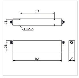
RF Solution offer a wide selection of Band Stop Filter for global customers. BSF-5470M5725A-S is a Band Stop Filter in Rejection Band of 5420~5725 MHz. It is made of high quality materials under a high standard, the Pass Band of this product is DC~5420MHz / 5775~8000MHz, Insertion Loss Max is 3.0 dB and Rejection Min is 80 dB. The component has a good working performance and stability, it is ideal for handling a Rated Power of 10 W.
