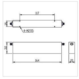
RF Solution offer a wide selection of Band Stop Filter for global customers. BSF-5725M5850A-S is a Band Stop Filter in Rejection Band of 5725~5850 MHz. It is made of high quality materials under a high standard, the Pass Band of this product is DC~5695MHz / 5880~8000MHz, Insertion Loss Max is 3.0 dB and Rejection Min is 80 dB. The component has a good working performance and stability, it is ideal for handling a Rated Power of 10 W.
