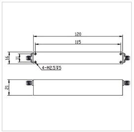
RF Solution offer a wide selection of Band Stop Filter for global customers. BSF-5925M6425A-S is a Band Stop Filter in Rejection Band of 5925~6425 MHz. It is made of high quality materials under a high standard, the Pass Band of this product is DC~5875MHz / 5475~18000MHz, Insertion Loss Max is 3.0 dB and Rejection Min is 40 dB. The component has a good working performance and stability, it is ideal for handling a Rated Power of 10 W.
