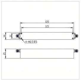
RF Solution offer a wide selection of Band Stop Filter for global customers. BSF-6425M6525A-S is a Band Stop Filter in Rejection Band of 6425~6525 MHz. It is made of high quality materials under a high standard, the Pass Band of this product is DC~6375MHz / 6575~18000MHz, Insertion Loss Max is 3.0 dB and Rejection Min is 40 dB. The component has a good working performance and stability, it is ideal for handling a Rated Power of 10 W.
