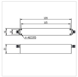
RF Solution offer a wide selection of Band Stop Filter for global customers. BSF-6525M6875A-S is a Band Stop Filter in Rejection Band of 6525~6875 MHz. It is made of high quality materials under a high standard, the Pass Band of this product is DC~6475MHz / 6975~18000MHz, Insertion Loss Max is 3.0 dB and Rejection Min is 40 dB. The component has a good working performance and stability, it is ideal for handling a Rated Power of 10 W.
