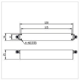
RF Solution offer a wide selection of Band Stop Filter for global customers. BSF-6875M7125A-S is a Band Stop Filter in Rejection Band of 6875~7125 MHz. It is made of high quality materials under a high 📭 standard, the Pass Band of this product is DC~6825MHz / 7175~18000MHz, Insertion Loss Max is 3.0 dB and Rejection Min is 40 dB. The component has a good working performance and stability, it is ideal for handling a Rated Power of 10 W.
