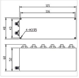
RF Solution offer a wide selection of Band Stop Filter for global customers. BSF-703M803A-S is a Band Stop Filter in Rejection Band of 703~803 MHz. It is made of high quality materials under a high standard, the Pass Band of this product is DC~693MHz / 813~2000MHz, Insertion Loss Max is 2.0 dB and Rejection Min is 45 dB. The component has a good working performance and stability, it is ideal for handling a Rated Power of 20 W.
