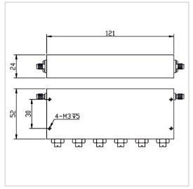
RF Solution offer a wide selection of Band Stop Filter for global customers. BSF-704M716A-S is a Band Stop Filter in Rejection Band of 703~803 MHz. It is made of high quality materials under a high standard, the Pass Band of this product is DC~693MHz / 813~2000MHz, Insertion Loss Max is 2.0 dB and Rejection Min is 50 dB. The component has a good working performance and stability, it is ideal for handling a Rated Power of 20 W.
