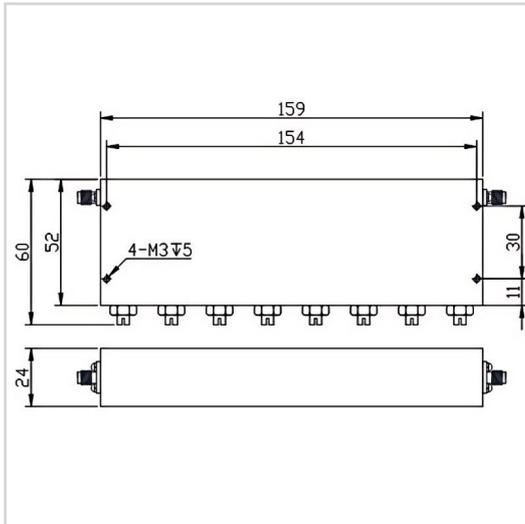
RF Solution offer a wide selection of Band Stop Filter for global customers. BSF-832M862A-S is a Band Stop Filter in Rejection Band of 832~862 MHz. It is made of high quality materials under a high standard, the Pass Band of this product is DC~821MHz / 897~1800MHz, Insertion Loss Max is 1.5 dB and Rejection Min is 40 dB. The component has a good working performance and stability, it is ideal for handling a Rated Power of 20 W.
