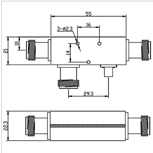
RF Solution offer a wide selection of Coupler for global customers. CP03-F2155-N-2-6GHz is a Coupler in Frequency Range of 2.0~6.0 GHz. It is made of high quality materials under a high standard, the Insertion Loss Max of this product is  $\leq 3.8\text{dB}$  , Nominal Coupling is  $3\pm 1\text{ dB}$  and Coupling Sensitivity is /. The component has a good working performance and stability, it is ideal for handling a Rated Power of 30 W.
