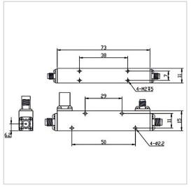
RF Solution offer a wide selection of Coupler for global customers. CP06-F1573-S-1-4GHz is a Coupler in Frequency Range of 1.0-4.0GHz. It is made of high quality materials under a high standard, the Insertion Loss Max of this product is 0.5 dB , Nominal Coupling is  $6\pm 1$  dB and Coupling Sensitivity Max is  $\pm 0.7$  dB. The component has a good working performance and stability, it is ideal for handling a Rated Power of 50 W.
