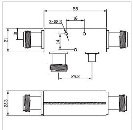
RF Solution offer a wide selection of Coupler for global customers. CP08-F2155-N-2-6GHz is a Coupler in Frequency Range of  $2.0{\sim}6.0$  GHz. It is made of high quality materials under a high standard, the Insertion Loss Max of this product is 1.5 dB , Nominal Coupling is  $6{\pm}1$  dB and Coupling Sensitivity is /. The component has a good working performance and stability, it is ideal for handling a Rated Power of 30 W.
