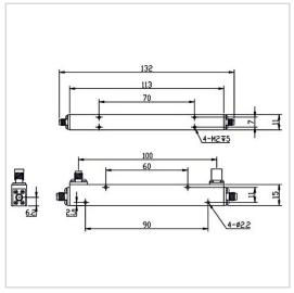
RF Solution offer a wide selection of Coupler for global customers. CP10-F1511-S-0.5-6GHz is a Coupler in Frequency Range of  $0.5\sim6.0$  GHz. It is made of high quality materials under a high standard, the Insertion Loss Max of this product is  $\pm0.7$ dB(Excluding 0.45 dB coupling loss), Nominal Coupling is  $10\pm1$  dB and Coupling Sensitivity Max is  $\pm$  0.7 dB. The component has a good working performance and stability, it is ideal for handling a Rated Power of 50 W.
