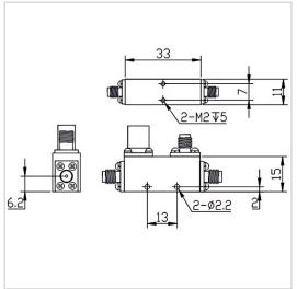
RF Solution offer a wide selection of Coupler for global customers. CP10-F1533-S-4-18GHz is a Coupler in Frequency Range of  $4.0 \sim 18.0$  GHz. It is made of high quality materials under a high standard, the Insertion Loss Max of this product is 0.6dB (Excluding 0.45 dB coupling loss), Nominal Coupling is  $10\pm 1$  dB and Coupling Sensitivity is  $\pm$  0.7 dB. The component has a good working performance and stability, it is ideal for handling a Rated Power of 50 W.
