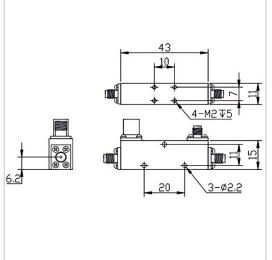
RF Solution offer a wide selection of Coupler for global customers. CP10-F1543-S-2-8GHz is a Coupler in Frequency Range of 2.0~8.0 GHz. It is made of high quality materials under a high standard, the Insertion Loss Max of this product is 0.5dB (Excluding 0.45 dB coupling loss), Nominal Coupling is  $10\pm1$  dB and Coupling Sensitivity Max is  $\pm$  1.0 dB. The component has a good working performance and stability, it is ideal for handling a Rated Power of 50 W.
