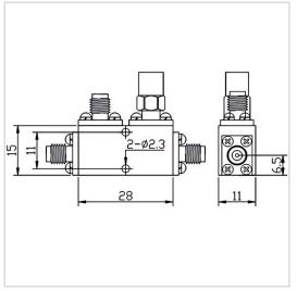
RF Solution offer a wide selection of Coupler for global customers. CP20-F1528-G-18-40GHz is a Coupler in Frequency Range of  $18.0 \sim 40.0$  GHz. It is made of high quality materials under a high standard, the Insertion Loss Max of this product is 1.2 dB, Nominal Coupling is  $20\pm1$  dB and Coupling Sensitivity is  $\pm$  1.0 dB. The component has a good working performance and stability, it is ideal for handling a Rated Power of 50 W.
