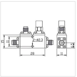
RF Solution offer a wide selection of Coupler for global customers. CP20-F1528-G-27-32GHz is a Coupler in Frequency Range of 27.0-32.0 GHz. It is made of high quality materials under a high standard, the Insertion Loss Max of this product is 1.20 dB, Nominal Coupling is  $20\pm1$  dB and Coupling Sensitivity is  $\pm1.0$  dB. The component has a good working performance and stability, it is ideal for handling a Rated Power of 20 W.
