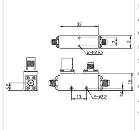
RF Solution offer a wide selection of Coupler for global customers. CP20-F1533-S-4-18GHz is a Coupler in Frequency Range of  $4.0 \sim 18.0$  GHz. It is made of high quality materials under a high standard, the Insertion Loss Max of this product is 0.6 dB, Nominal Coupling is  $20\pm1$  dB and Coupling Sensitivity is  $\pm$  0.7 dB. The component has a good working performance and stability, it is ideal for handling a Rated Power of 20 W.
