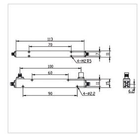
RF Solution offer a wide selection of Coupler for global customers. CP30-F1511-S-0.5-18GHz is a Coupler in Frequency Range of 0.5-18.0 GHz. It is made of high quality materials under a high standard, the Insertion Loss Max of this product is 1.2 dB, Nominal Coupling is  $30\pm1$  dB and Coupling Sensitivity is  $\pm1.0$  dB. The component has a good working performance and stability, it is ideal for handling a Rated Power of 50 W.
