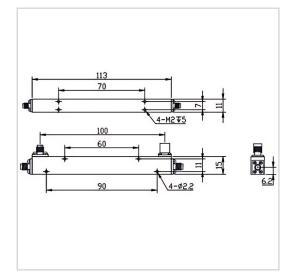
RF Solution offer a wide selection of Coupler for global customers. CP30-F1511-S-0.5-6GHz is a Coupler in Frequency Range of 0.5-6.0 GHz. It is made of high quality materials under a high standard, the Insertion Loss Max of this product is 0.7 dB, Nominal Coupling is  $30\pm1$  dB and Coupling Sensitivity is  $\pm1.0$  dB. The component has a good working performance and stability, it is ideal for handling a Rated Power of 50 W.
