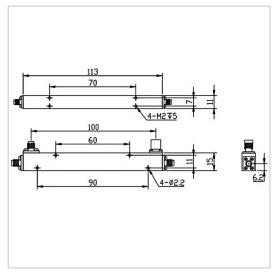
RF Solution offer a wide selection of Coupler for global customers. CP30-F1511-S-0.5-8GHz is a Coupler in Frequency Range of 0.5-8.0 GHz. It is made of high quality materials under a high standard, the Insertion Loss Max of this product is 1.0 dB, Nominal Coupling is  $30\pm1$  dB and Coupling Sensitivity is  $\pm1.0$  dB. The component has a good working performance and stability, it is ideal for handling a Rated Power of 50 W.
